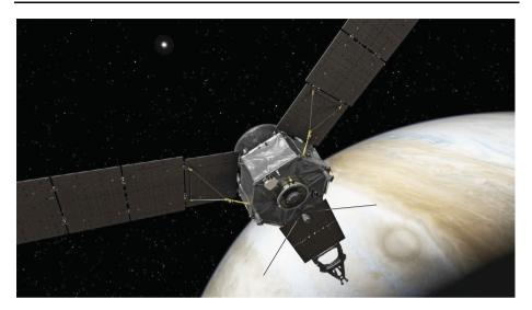
Fig. 15 Juno with Waves electric antenna deployed from the aft flight deck. The sensitive axis is perpendicular to the solar panel containing the magnetometer boom (spacecraft x axis) and the spin (z) axis
