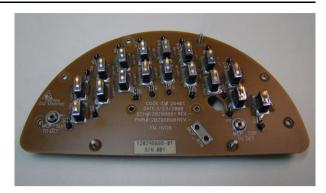
Fig. 17 JADE-E Charge Amplifier Board
