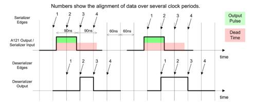
Fig. 20 JADE-E Digital Board timing diagram
