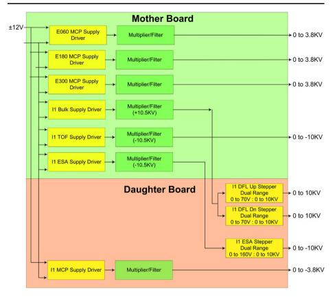
Fig. 38 HVPS Board 2 block diagram
