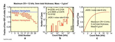
**Fig. 43** For JADE-I: (a) fraction of time that background count rate are below 6 kHz for each of Juno's orbits in the northern and southern hemispheres; (b) number of cases vs. estimated background count rate for JADE-I; and (c) integral fraction of time above various count rates
