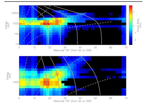
Fig. 82 Energy-TOF spectrograms for two different sweep tables. Overplotted on the data are curves of constant M/q (solid lines) and constant incident velocity (dashed lines). The top panel shows data for sweep table 1, which covers from 10 eV-40 keV (the same energy steps as used during HRS mode and shown in Fig. 81). The bottom panel shows data for sweep table 2, which covers the typical solar wind energies of 0.3-8 keV
