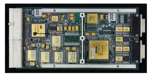
Fig. 30 Instrument Processor Board (IPB)
