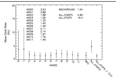
Fig. 68 Dark rate observed in the JADE-I sensor during flight calibration. The mean dark rate for each anode is indicated by the horizontal line, and the vertical line is  $\pm 1\sigma$
