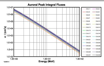
Fig. 41 Peak integral fluxes from the auroral region for all orbits (note that orbit numbering here starts with the first complete 11-day orbit). Since the auroral region is in L-shells > 6, the JPL-DG model was used to calculate integral fluxes. The SwRI-DSC model was applied only to orbit segments where L < 6
