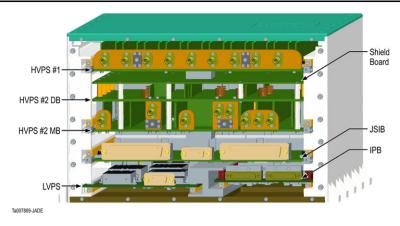
Fig. 29 The JADE Electronics Box
