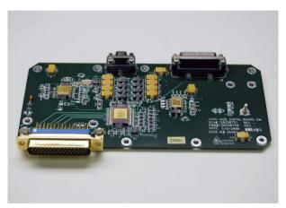
the various adjustable parameters of the A121. The threshold is fixed at  $3 \times 10^6$  electrons. The pulse width is set to 90 ns and the dead-time at 180 ns.
