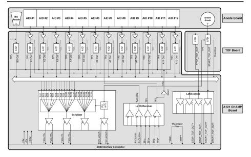
Fig. 23 Overview of the JADE-I Charge Amplifier and TOF Boards
