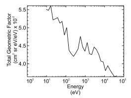
The geometric factor for JADE-I was determined through particle ray tracing based on SIMION modeling where  $2.6 \times 10^6$  ions were launched into the JADE-I electro-optics for each of the 32 nominal ESA voltages settings; it was also measured directly in calibration using 10 and 40 keV ions of 3 different species. Figure 64 shows geometric factor assuming 100 % foil and grid transmission and detection efficiency.
