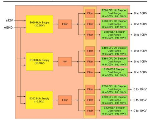
Fig. 37 HVPS Board 1 block diagram
