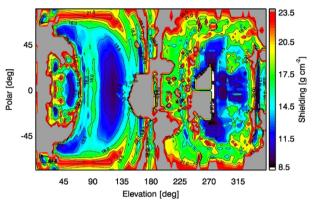
maximum rate on the worst and best anodes was 2.2 kHz and 2.0 kHz, respectively, showing that the shielding is well-distributed and optimized for JADE-E.
