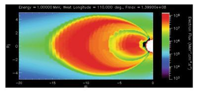
Fig. 40 Differential fluxes from the SwRI-DSC physical model for L < 6 and the JPL-DG model for L > 6. The differences between the physical model and JPL code for L < 6 are significant only in relation to the differential fluxes; the simulation results from the two models are similar in terms of the integral flux
