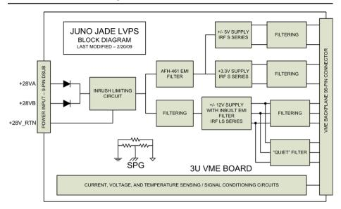
Fig. 33 LVPS block diagram
