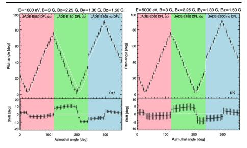
Fig. 9 Simulations of pitch-angle deflection of (a) 1 keV and (b) 5 keV electrons after passing through the ESA of the JADE-E sensor in an external magnetic field strength of  $B_X = 2.25$  G,  $B_Y = 1.3$  G,  $B_Z = 1.5$ , and B = 3 G. The *white curve* is undeflected pitch angle. The *bottom panels* show the angular shift
