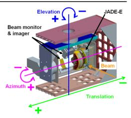
JADE-I was calibrated in the Southwest Research Institute ion instrument calibration facility (see Appendix in McComas et al. 2009), which was totally refurbished and expanded into a world-class facility starting in late 2000. In order to fully and properly calibrate the three JADE-E sensors, we designed, built and validated a completely new electron calibration facility. The details of this new facility are described in the Appendix of this paper.
