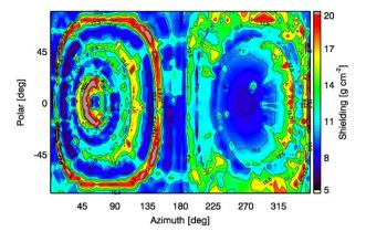
Fig. 46 Rectangular projection of the JADE-E radiation shielding thickness viewed from Anode 8
