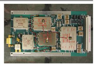
The IPB responds to spacecraft commands, transmits low-rate Science and Housekeeping telemetry, and transmits high-rate, synchronous Burst Mode Science data. Through the JSIB, the IPB controls the sensors and reads back telemetry data collected. The data is then formatted into packets and transmitted to the spacecraft.
