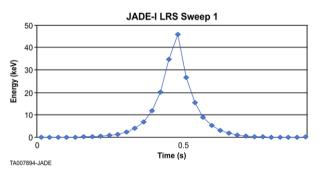
Jupiter, while the second covers the energy range from 350 eV to 7.7 keV to be used during cruise to measure the solar wind; this energy range will cover the most probable solar wind velocities (Gosling 2007). The third table covers energies from 125 eV to 45 keV, and the fourth, energies from 5 eV to 25 keV. The deflector supplies do not sweep in this mode.
