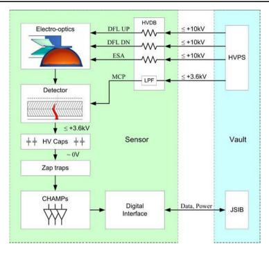
Fig. 14 JADE-E Sensor Electronics block diagram
