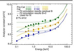
due to relativistic effects is necessary to account for the dependence on the energy of the analyzer constant. The analyzer constant can be related to the equation of motion in the analyzer.
