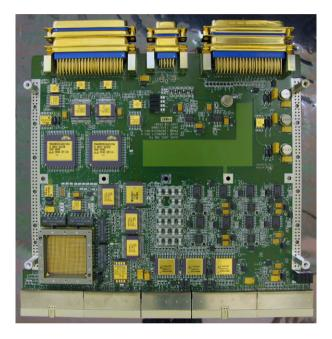
Test pulsers to all of the sensors can be generated by the JSIB so that the amplifiers in each of the sensors can be checked at any time. Various rates and combinations can be selected. In the case of JADE-I various TOFs are also selectable.
