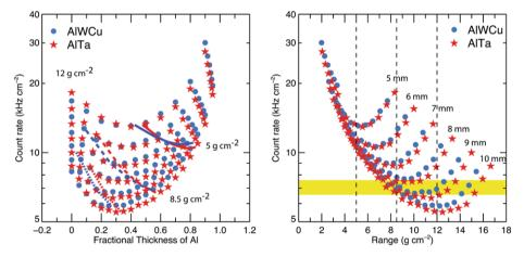
Fig. 42 Estimated MCP count rate plotted vs. (a) the fractional thickness of Al, and (b) the stopping power of the graded-Z shield
