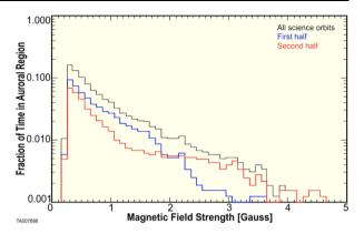
During the course of the mission, Juno traverses auroral regions where the magnetic field strength exceeds 3 G. Under these conditions, the gyroradii of low-energy (<5 keV) electrons are comparable to the scale size of the ESA; consequently, measurements from the ESA-based sensor are significantly aberrated. For instance, using the simple relation
