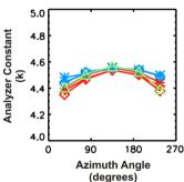
The calibration data agrees well with the model results. In Fig. 60 the measured values for the flight unit for 10 and 40 keV are plotted for three species: He<sup>+</sup> (stars),  $N_2^+$  (diamonds), and Ar<sup>+</sup> (crosses). The measured values differ by  $\sim$ 5 % from the modeled values.
